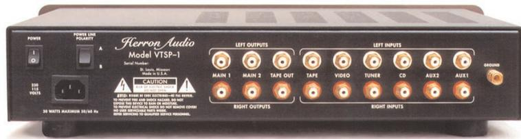
The rear panel was designed for flexibility and ease of access to less-frequently used functions. The high precision RCA input jacks are heavily gold-plated to minimize signal-degrading corrosion. The special insulation material in the RCA connectors maintains purity of the signal from the input cable into the unit.
