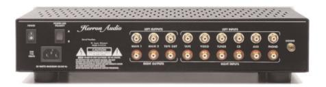
The rear panel was designed for flexibility and ease of access to less-frequently used functions. The high-precision RCA input jacks are gold-plated to minimize signal-degrading corrosion. The special Teflon insulation material in the RCA connectors maintains purity of the signal from the input cable into the unit.
